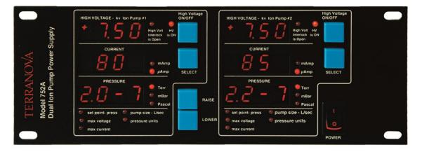
The Terranova Model 752A Ion Pump Control Unit is designed to supply operating power to two sputter ion pumps and to display the voltage, current and pressure independently for each. It is designed to start and operate pumps of 60 l/s and smaller and to operate larger pumps of any size at lower pressures.
