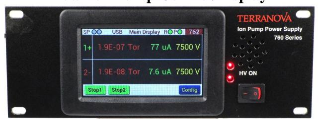
The Terranova Model 762 Ion Pump Control Unit is designed to supply operating power to two sputter ion pumps and to display the voltage, current and pressure independently for each. It is designed to start and operate pumps of 60 l/s and smaller and to operate larger pumps of any size at lower pressures.
