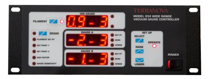
The Terranova Model 934 displays pressure from one 563-type Bayard-Alpert ion gauge (for high- and ultra-high vacuum environments) and two low-vacuum gauges (either 531-type thermocouple gauges or convection gauges, depending upon the purchased configuration).
