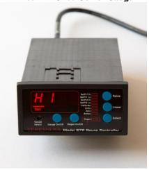
The Terranova Model 970 Vacuum Gauge Controller displays pressure from 5x10-10 Torr to 1500 Torr, as measured from the MKS/HPS Series 910, 925C, 972, 979B; Inficon BPG-400 Combi Gauge and other modular vacuum transducers
