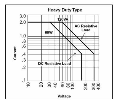
For resistive loads maximum current varies from 2 amps at 30 VDC (60 VAC) downward to 0.4 amps at 150 VDC (300VAC).
