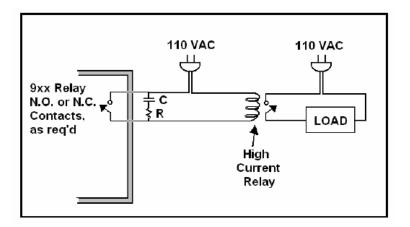
To calculate the values of C and R for the "snubber' circuits, the equations below give some guidance.
