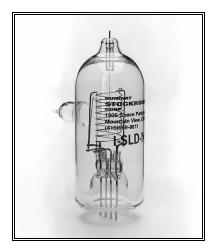
Glass Ionization Gauge - Sealed Reference |Tube Duniway Stockroom Part Number: I-SLD-N
