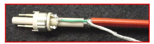
Figure 2: Part g, with coax and low voltage conductors installed.
