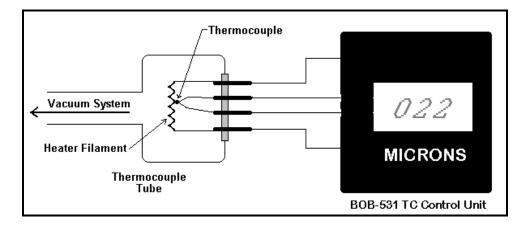
Figure 1: Diagram of Thermocouple Tube and Control Unit
