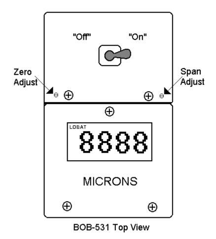
Figure 3: Top View Showing Adjustments, Low Battery Indicator and Power Switch
