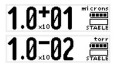
The Numeric display shows the currently configured units, in these examples, the vacuum pressure units are 'microns' or 'Torr'. Below the units indicator are the battery, vacuum pressure, and vacuum system analysis indicators.
