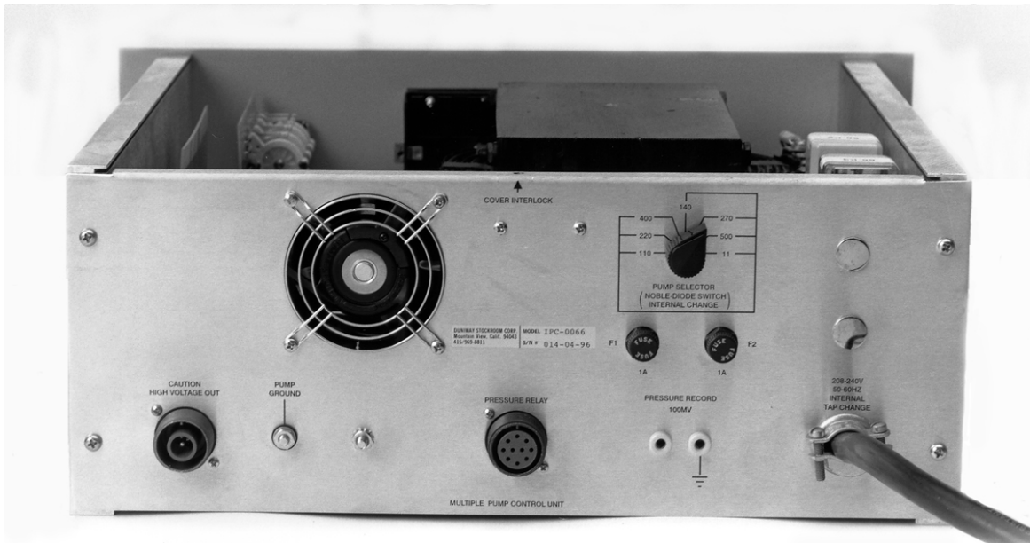
Figure 5: Rear Control Panel
