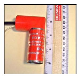
The R-style (R for Right-angle) Ion Pump High Voltage Connector attaches to the Varian-style HVFT-5143 Ion Pump High Voltage Feedthrough. It is intended for applications where space is limited for the pump connector. Where the V-Style connector (Duniway Part Number V-100-X) requires almost 7 inches of clearance from the connector face, the R-style requires just over 3 inches clearance from the same point (lower face of connector in above photo).
